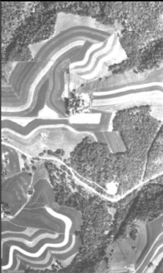
Aerial photographs of a selected region of Coon Creek basin. Picture on right from 1934 shows rectangular fields and gullies across fields from overland flow of water. Picture on left of the same area in 1967 planted in contour strips to reduce soil erosion.
